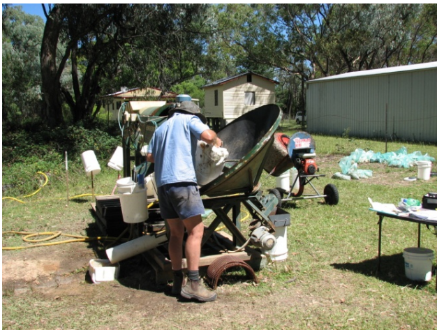
Figure 2: Testing Karaula Lead alluvial samples in the cone concentrator:
