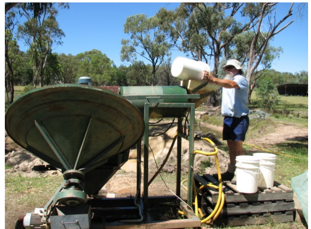
Figure 2: Testing Karaula Lead alluvial samples in the cone concentrator:
