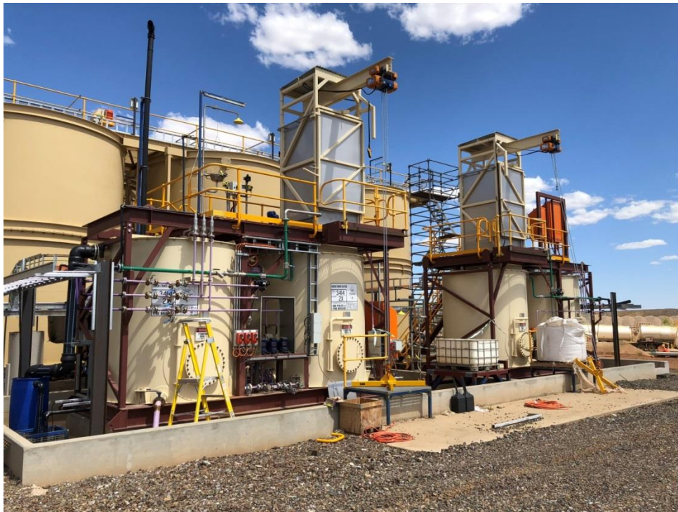
Lorena Gold Mine – Processing Plant: Lime and acid modules.
