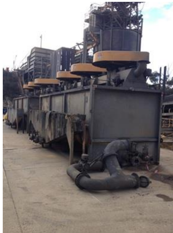
Photo 1: Flotation cells removed from Beaconsfield Plant for transportation to Lorena
